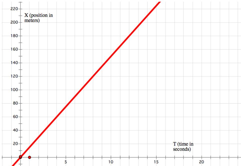
This motion map indicates that as time goes on the object gets further and further away from the point of origin. The change is consistently 15 meters for every one second
