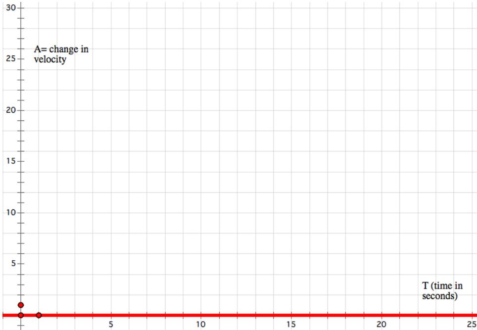
Acceleration is a change in velocity. Since the velocity is constant there is no **acceleration**.
