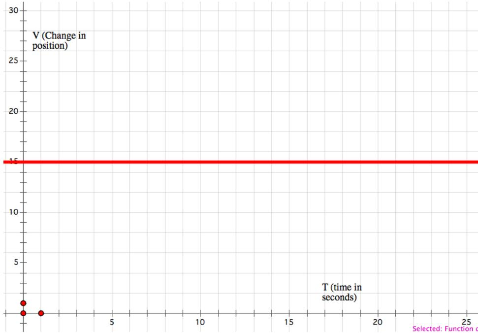
The line is at 15 on the y axis because over time the vehicle is traveling constantly at 15.
