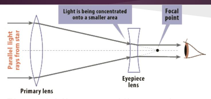
This <u>convex</u> spherical lens (called the primary lens) collected and concentrated the light ... ... and this <u>concave</u> eyepiece lens made the concentrated light rays parallel again.
