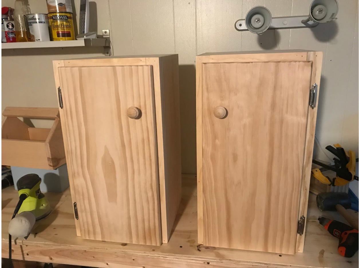
These are the two Cabinets I produced for my capstone. They were built with Pine softwood and assembled using wood jointing.
