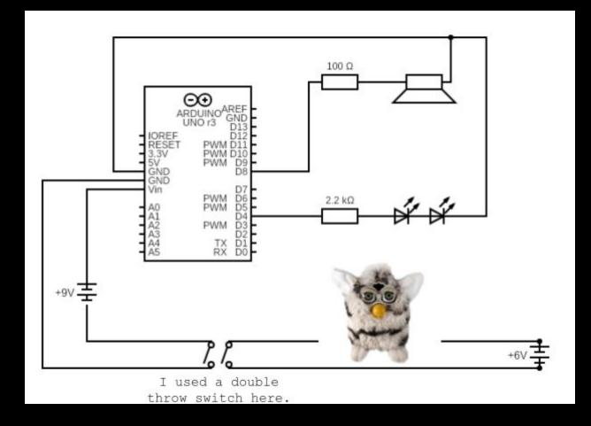
To make the schematic, I used a website called circuit-diagram.org. It's very simple and makes downloading the schematic easy. Most of the electronics design for this came from the Arduino website, as well as what I knew about powering Jill. I didn't include the details on what's happening inside of Jill, since you can reference the Furby schematic that can be found in the resources section.
